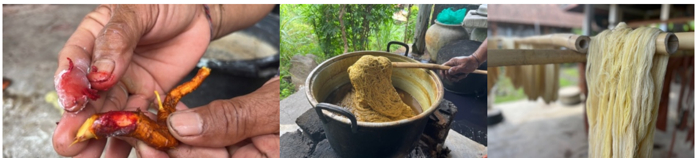
Fig 8. The procedure of picking yellow ginger, boiling threads, mixing and drying, on Bali in Seraya-Kerajinan Tenun.
