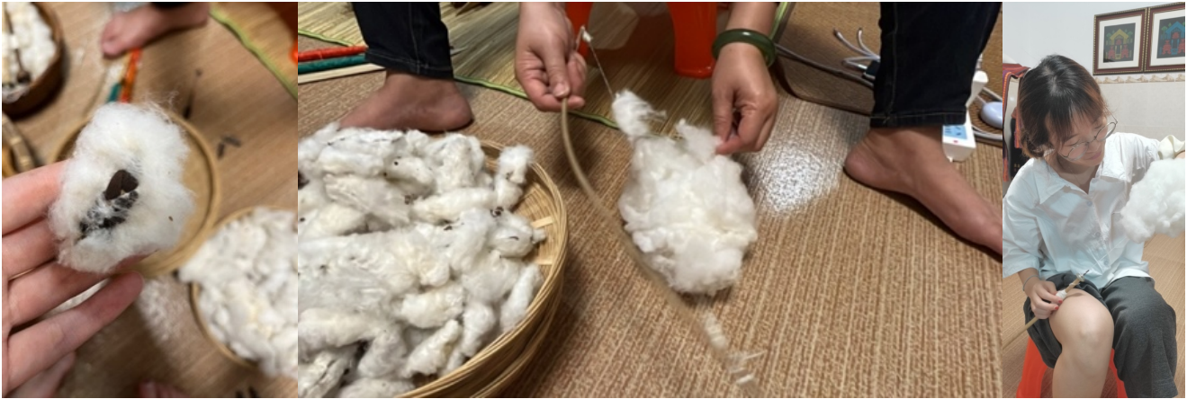
Fig 5. The procedure of removing cotton seeds, fluffing the cotton, and spinning the fibers on Hainan
