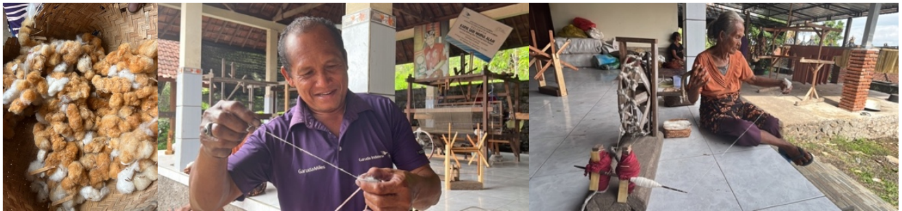
Fig 6. The procedure of removing cotton seeds, fluffing the cotton, and spinning the fibers Bali in Seraya-Kerajinan Tenun
